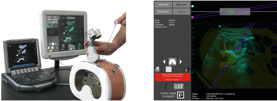
Fig. 1. (a) Clear Guide SCENERGY system, with touchscreen computer, hand-held SuperPROBE (ultrasound probe with mounted Optical Head), connected to a standard ultrasound system. (b) User interface in Fusion Mode, with registered US and CT and overlaid tracked instrument path.
