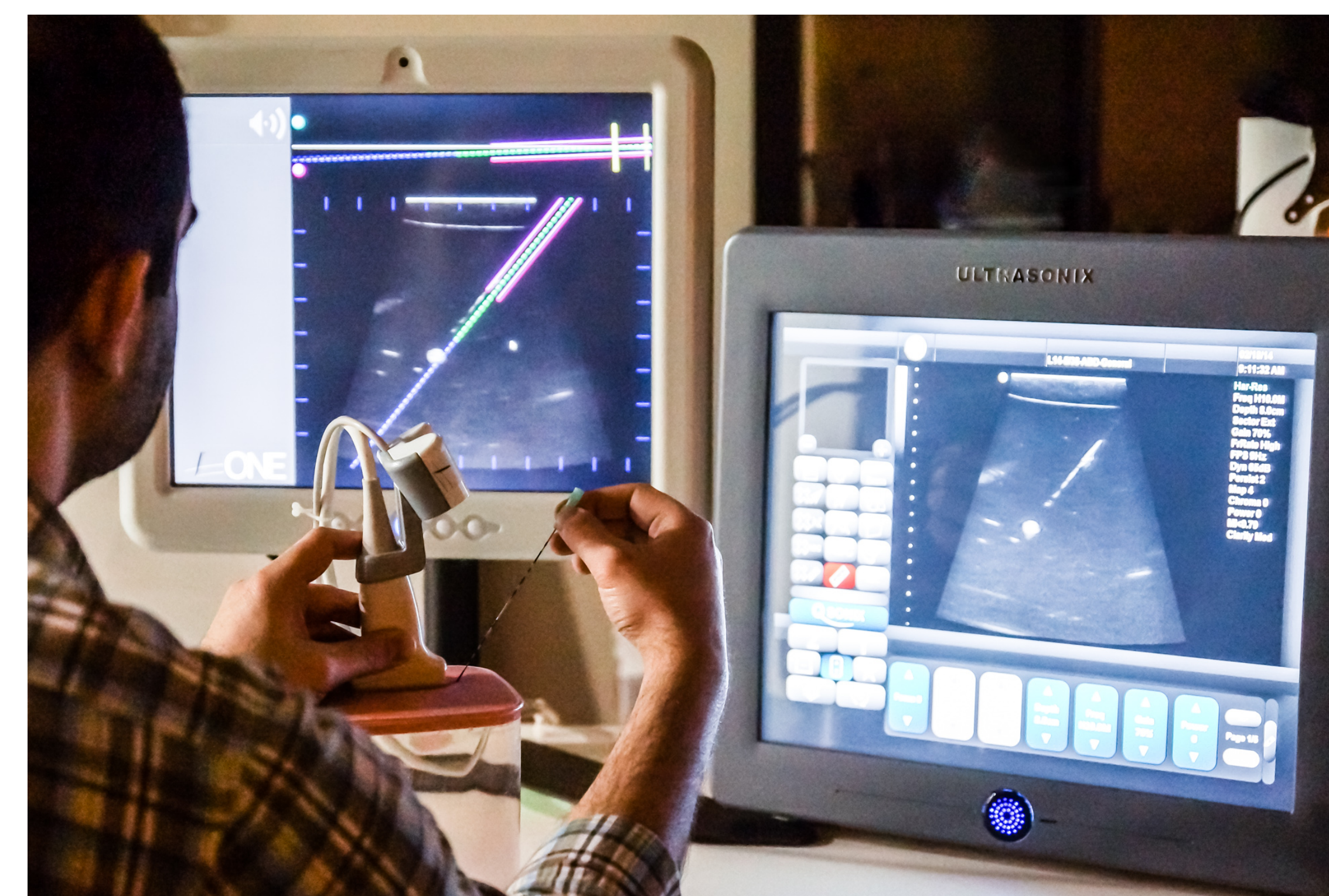
Fig. 2: Insertion depth tracking (magenta lines) on guidance display (left screen)
