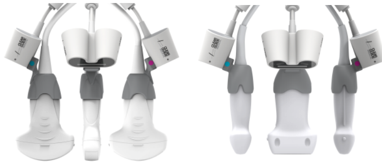
Figure 2: Optical Head tracking hardware on standard ultrasound probes (left: in-plane, right: out-of-plane configuration)
