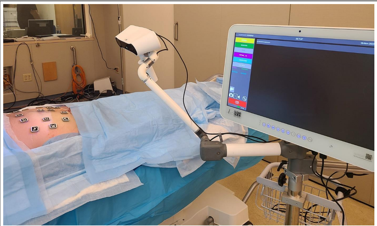
Figure 1. Augmented reality LUMENA system for MRI-guided needle-based interventions. A panel PC and an articulated arm with an optical head mounted on an MR-safe cart. The system is designated MR conditional and designed for continuous operation in the MRI environment (<300 Gauss for the optical head and <100 Gauss for panel PC).
