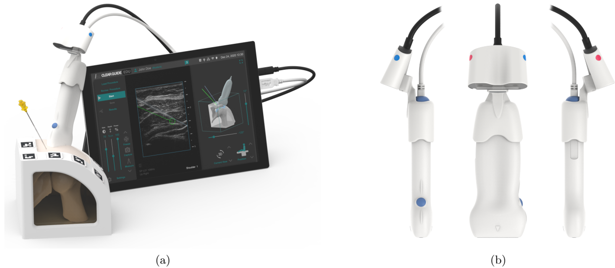
Figure 1. Left: The EDU system. Right: EDU SuperProbe: linear ultrasound probe with optical head.
